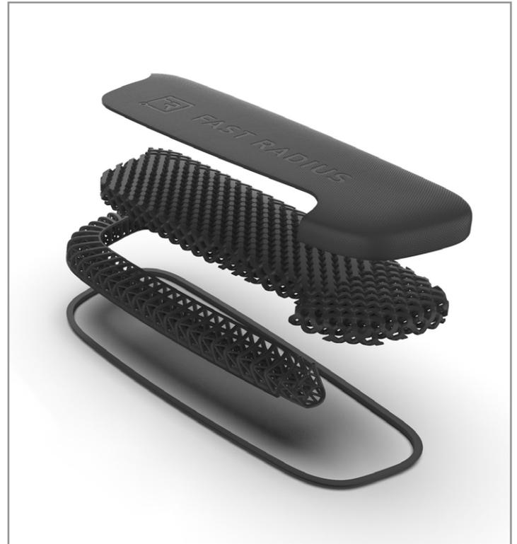
might interact with the cap. Although each zone was designed separately, Carbon's DLS technology allowed the entire arm cap to be printed as one cohesive part using EPU 41, a material that is both flexible and conforming. And the use of lattices reduced material usage by up to 70% without sacrificing performance.
